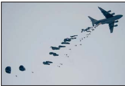
C-17 airlifter carrying out a long distance air drop of humanitarian daily rations.
