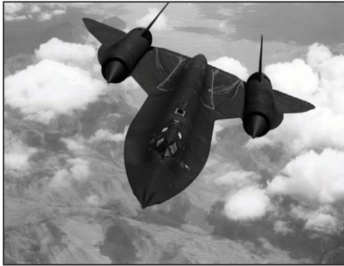
The Lockheed SR-71 Blackbird strategic reconnaissance aircraft, first employed during the Vietnam War. A marvel of technology, it outperformed all of the other military aircraft of its time, attaining altitudes above 85,000 feet and speeds of nearly Mach 3.5.
